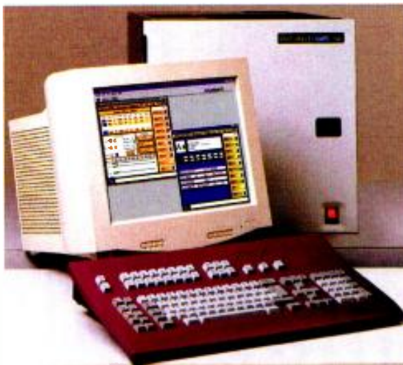
(Right) The Chyron Infinit character generator remains the standard by which all other character generators are judged in many circles, particularly the live news or sports production environment.
